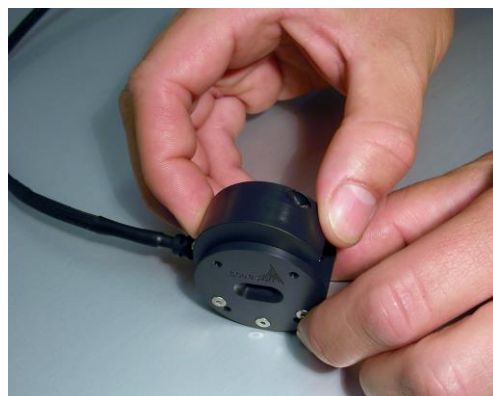
Figure 3. Oven top replacement
